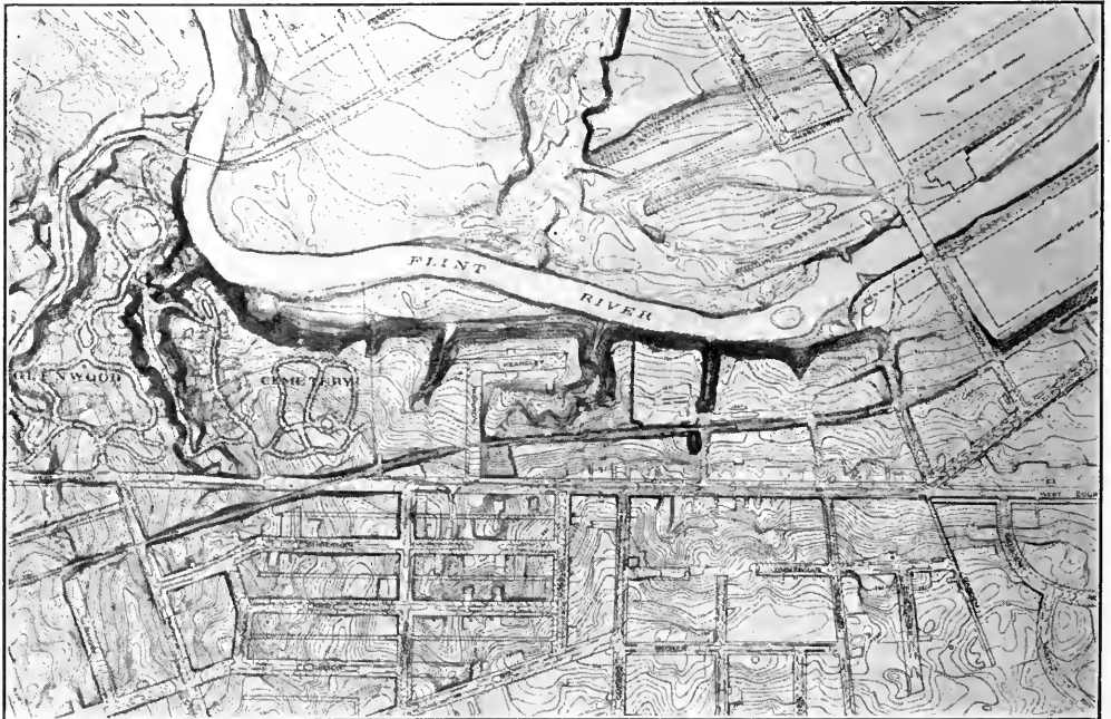
TOPOGRAPHICAL MAP OF A PART OF FLINT, MICH., USED IN SEWER DESIGN
